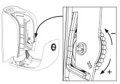
Roll Brake Settings Turn upwards to decrease roll breaking Turn downwards to increase
